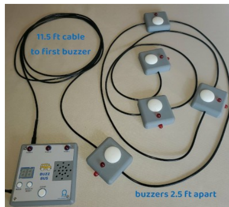
Figure 1: Buzz Bus setup showing one 5-buzzer chain plugged into Team A connector
